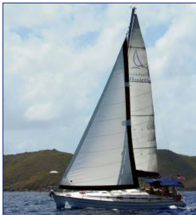
This sloop rig has a high aspect ratio main sail along with a fin keel, perfect for light air.
