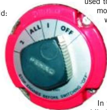
Using position number 1 while motoring, only the starting battery is charged. Under sail, battery number 1 provides power to the electrical system if left in this position. This is not recommended since battery number 1 should be kept fully charged.
