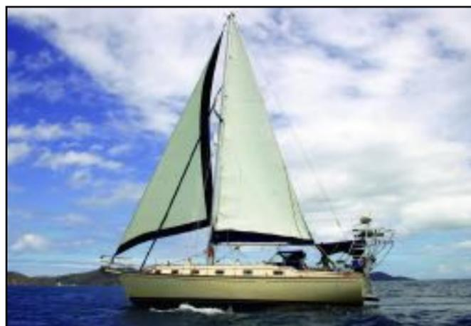
*The Island Packet's cutter rig offers multiple sail plans and its full keel provides additional stability in heavy winds.*
