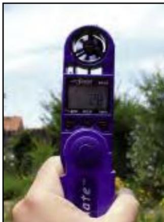
Hold up the WindMate 200 to check temperature, wind speed, heading and more.
