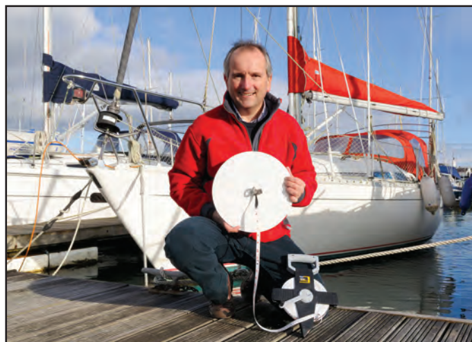
(Above) Dr. Richard Kirby, project leader, holds a Secchi Disk. This disk (also shown below) is being used in a unique, citizen science study along with a free mobile phone app called Secchi (below and left) to conduct a vital global study of the sea's phytoplankton.
